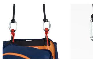
The two connections should be made using screw-lock karabiners with a breaking strength of at least 1,400 kg. It is important to verify that the length of the bridle is sufficient to position the reserve parachute inside the harness pocket, and that there is sufficient play to enable the parachute to be taken out of the pocket without causing the reserve parachute deployment bag itself to open during extraction.
